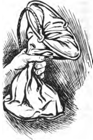
Fig. 3. A BUCKET THROTTLED FOR SOFT GROUND.
